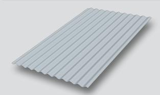
The minimum roof pitch for Corrugate is 8 degrees, and if end lapped, the pitch should be 10 degrees to ensure proper water drainage.
