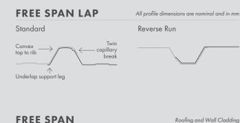
Dimensioned Drawing of Free Span
