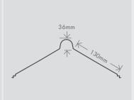
Our roll top ridge capping prevents rain or water from entering the house via the apex of the roof. It also prevents rainwater from penetrating the lower levels of a roof, which can damage the entire roof structure. Freeman Roofing ridge capping comes in a full range of colours and is made from genuine NZ made Colorsteel®
