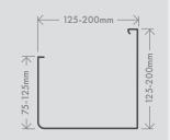
Quad gutter provides an attractive take on the traditional quarter round gutter, providing a bigger water flow capacity for higher rainfall areas. Quad's gently curved front and strong swaging offer a unique blend of traditional & modern looks.
